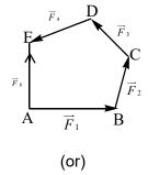
If a number of coplanar forces are acting simultaneously at a point keep the particle in equilibrium, these forces can be represented as the sides of a polygon taken in order both in magnitude and direction.
