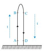
5. If an object is dropped (means initial velocity is zero) from Height h. Its speed on reaching ground is  $v = \sqrt{2gh}$  and
