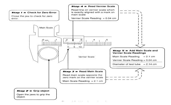
a) <u>Positive zero error :</u> If the zeroth division of the vernier scale is to the 'right' of the zeroth division of the main sacle, then the error is said to be positive and the correction is negative.
