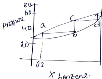
b → c → No change in mole fraction, vapour pressure increases → So it is condensation.
