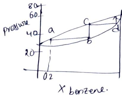
b - c  $\rightarrow$  No change in mole fraction, vapour pressure increases  $\rightarrow$  So it is condensation.
